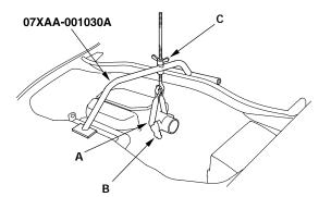
NOTE: For '02 model, replace the cable eye/bolt assembly (A) on the engine support hanger with T/N 07ZAA-S0XA100.
